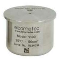
The Density of a coating should remain constant from batch to batch. Also known as Density Cups or Specific Gravity Cups, Pycnometers are used to determine the specific weight per unit volume of a liquid at a given temperature.
